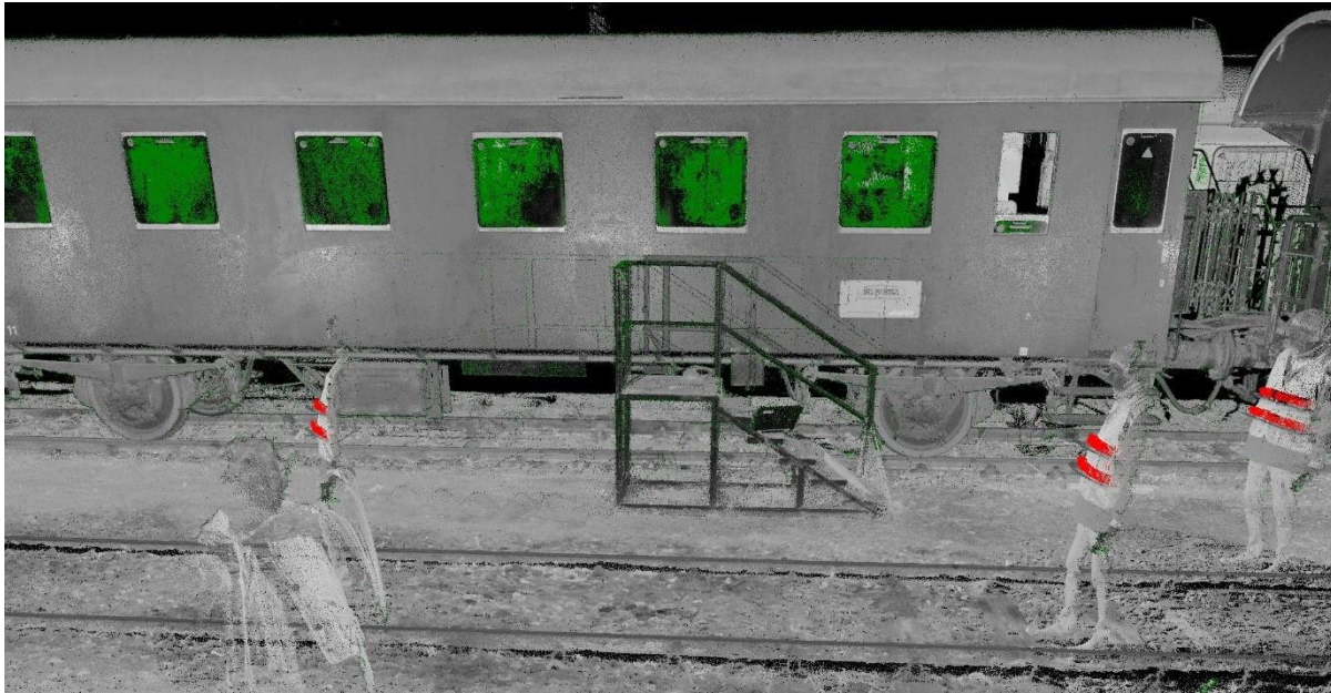
Figure 10: Red dots indicate highly reflective targets (here: reflective stripes on the guards), green dots indicate weakly reflective targets.
