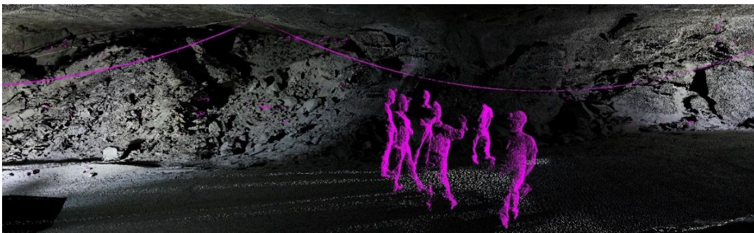
Figure 14: Targets moving in the point cloud (people and lines) were detected and highlighted (purple)
