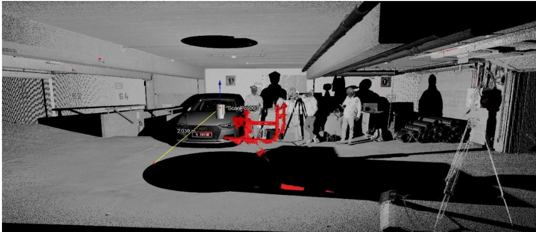
Figure 13: The laser scanner is mounted on a wheeled robot. It also measures parts of the robot itself. These points can be marked and removed with a distance filter (0 - 1.8 m), aka "range gate."
